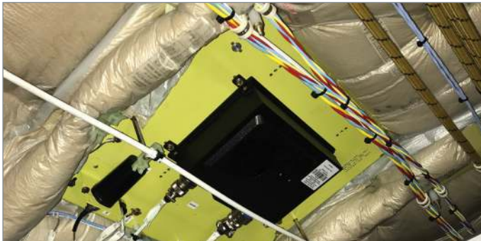
Wireless IFE system (Airbus A320 shown)
