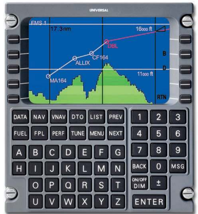
The Profile View shows terrain under the projected flight path. VNAV waypoints from the flight plan can be shown at their respective assigned altitudes. Look Ahead conflict advisories are depicted with a white threat symbol.
